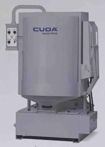
The Cuda 2530 is the smallest in the front-load automatic parts washer models and is smaller than many solvent tanks. Featuring a turntable diameter of 25-inches, working height of 30-inches, and load capacity of 500 lbs. The 2530 Series is equipped with a 3 HP vertical seal-less pump producing 50 GPM at 45 PSI. The Cuda 2530 front load aqueous parts washer is used in many applications from automotive, trucking, amusement parks to ski areas.
