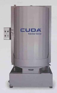
The Cuda 3648 features a turntable diameter of 36-inches, working height of 48-inches, and load capacity of 2500 lbs. The 3648 Series is equipped with a 7.5 HP vertical seal-less pump producing 150 GPM at 50 PSI, and has a 113-gallon sump capacity. It also includes upgraded features such as a more durable control panel, easier to replace handle, stainless steel sump covers, and external plumbing making it the easiest to maintain Cuda yet!
