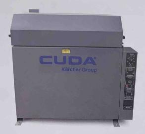
The newest addition to the Cuda top load line-up, the SJ-15 uses a patented spray wash technology which eliminates the need for a drive motor, gears and pulleys. Using a water-propelled spray arm with 23 nozzles that spin around a stationary parts basket, parts are hit from every angle while being cleaned. It has a 350-lb. load capacity, and a basket dimension of 32" x 21", 90 gallon sump capacity, 3 HP pump motor delivering 37 GPM @ 30 PSI.
